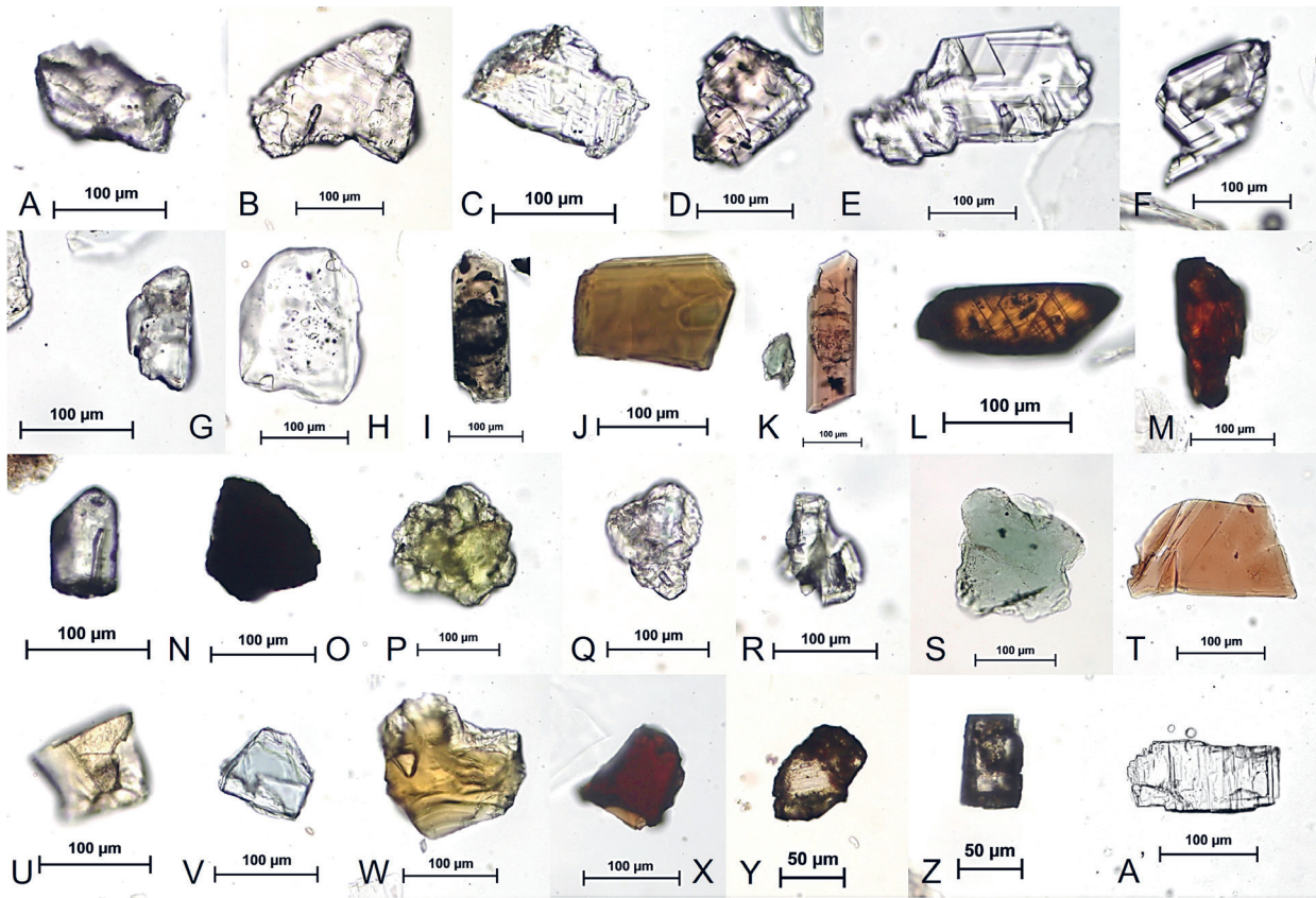
Figure 4. Heavy mineral association of the Upper Miocene sandstones from the Sava and Drava depressions. A – Anhedral garnet with conchoidal fractures, B-F – Garnet grains showing small to large-scale etch facets due to advanced dissolution, G & H – Apatite grains, I-K – Tourmaline grains, L & M – Rutile grains, N – Zircon, O – Opaque mineral grain, P – Epidote, Q – Clinozoisite, R – Zoisite, S – Chlorite, T – Biotite, U – Titanite, V – Chloritoid, W – Staurolite, X – Chromite, Y – Brookite, Z – Anatase, A' – Kyanite.
