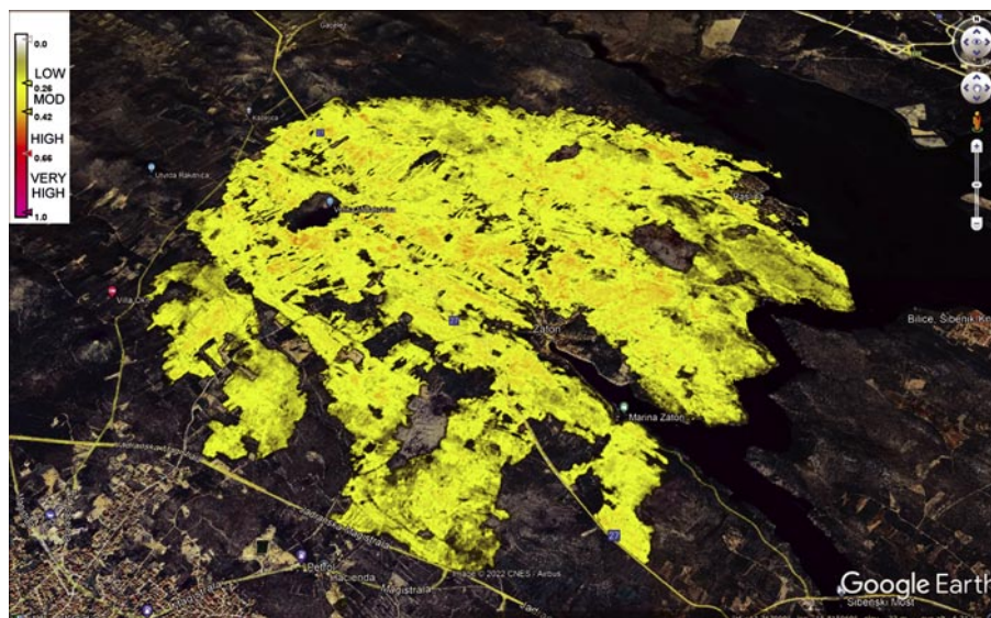
Figure 11. Burn categorization obtained using the difference bi-Normalized Burn Ratio ( dbNBR ) instead of RBR (Fig. 8), the detected burned area is identical in both cases with the expected lower categories of the burned areas (see text).
