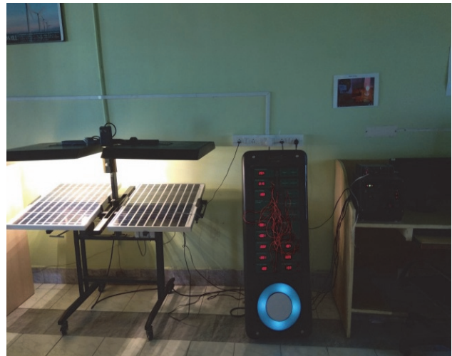
Figure 10 Experimental setup of parallel connection of PV modules with DC load
