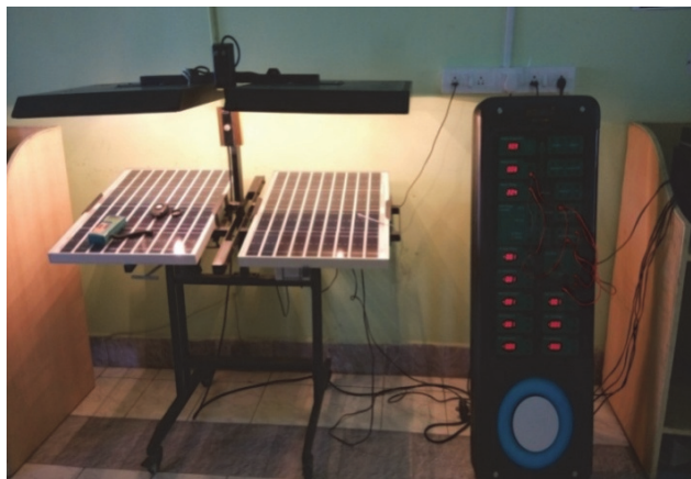
Figure 1 Experimental setup of standalone PV system
