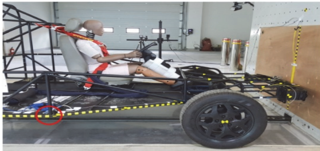
Figure 5 Equipment location of roadster acceleration sensor
