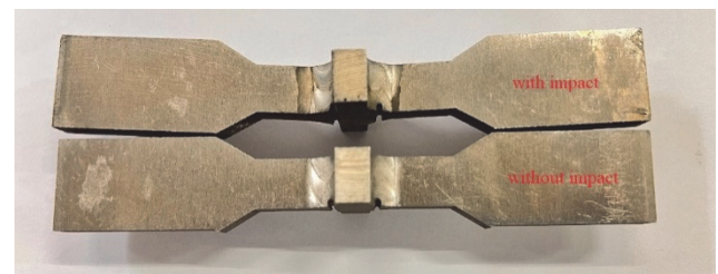
Figure 5 Impacted welded joint
