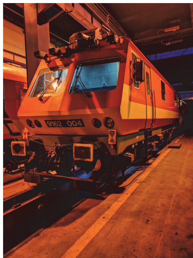
Figure 1 FMK-004 Track measuring car
