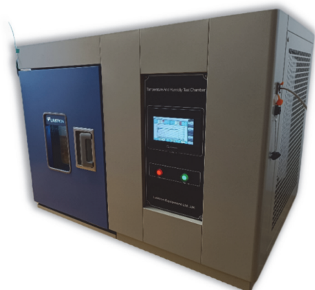
Figure 2 Climate chamber - Labtron temperature and humidity test chamber rLTHC-A10
