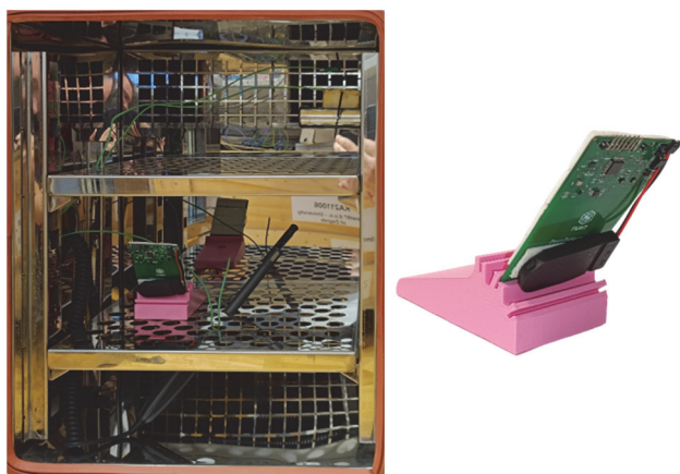
Figure 5 Experimental setup of the control devices and the smart sticker sensors for measuring the temperature and relative humidity data points values
