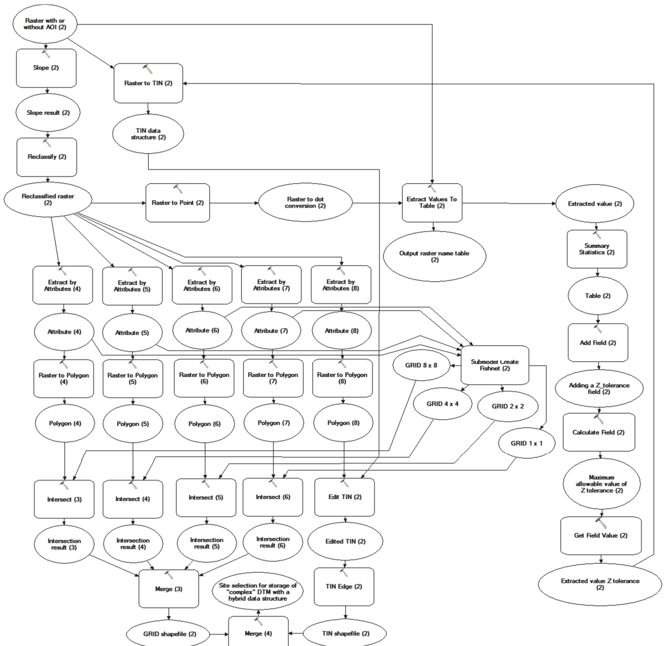
Figure 10 Submodel - complex DTM with a hybrid data structure
