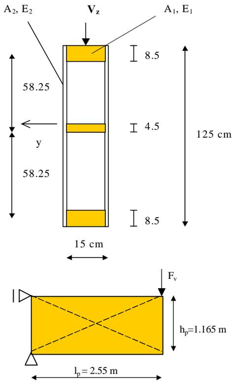
Fig. 3 Scheme of the static system and of the composed cross section of the test samples
