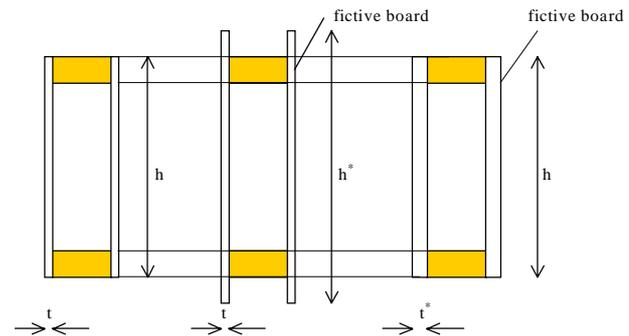
Fig. 2 Mathematical models: a) Normal panel (without reinforcement); b) Panel with a fictive height; c) Panel with a fictive thickness
