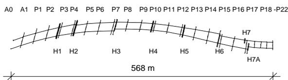
Fig. 2 Plan view of the superstructure of the Downtown viaduct in Las Vegas
