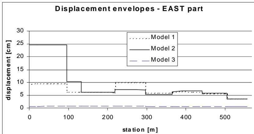
Fig. 11 Envelopes of the superstructure displacements obtained with three different models of the viaduct
