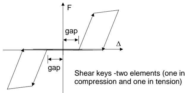
Fig. 9 Model of the shear keys
