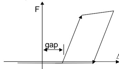
Fig. 7 Model of elements representing restrainers
