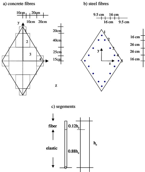
Fig. 4 Model of the “diamond” columns
