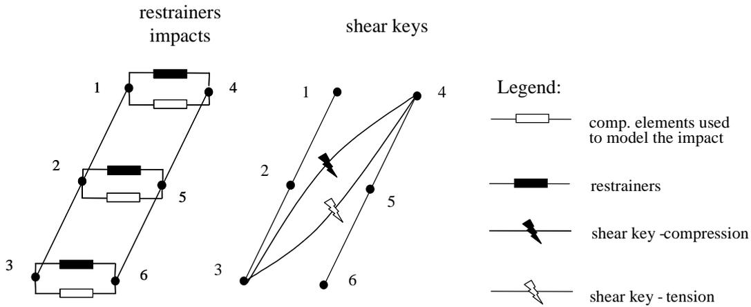
Fig. 6 Scheme of the transverse hinge - type 1
