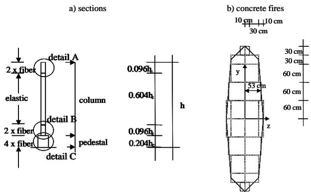
Fig. 5 Model of the columns in the single column piers
