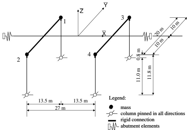
Fig. 12 An idealised structure, similar to the segments of the analysed viaduct
