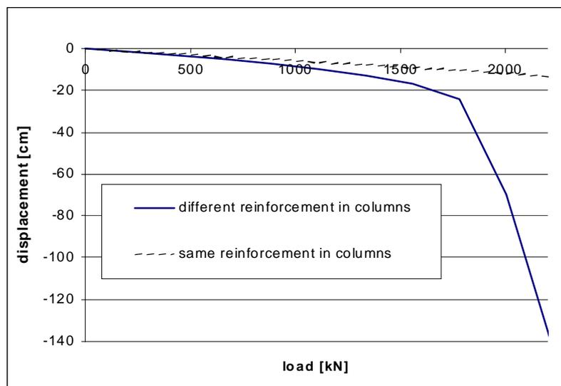
Fig. 13 Displacements of structures with different column reinforcement
