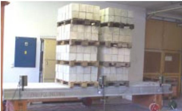
Fig. 3 Central loading of the plate after step 4
