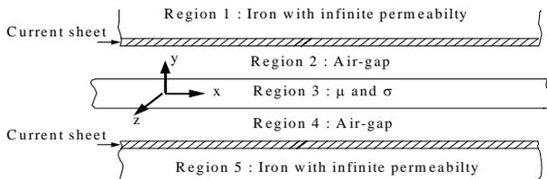
Fig. 1 Model of double-sided linear induction motor
