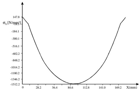
Fig. 12 Distribution of normal stress  $\sigma_x$  as a function from distance  $x$
