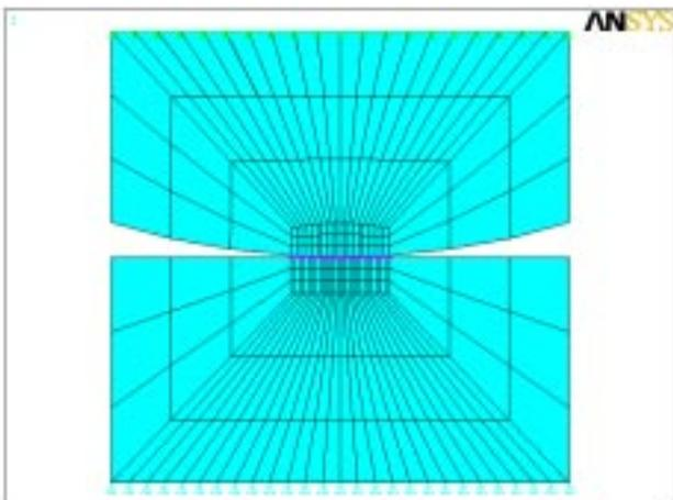
Fig. 4 Finite elements of the cylinder and plate
