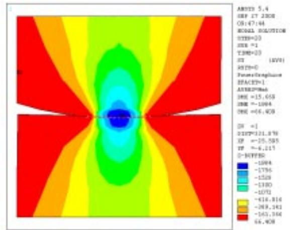
Fig. 6 Distribution of normal stress in direction of axis  $x$
