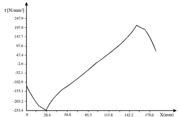
Fig. 11 Distribution of shear stress  $\tau$  as a function from distance  $x$
