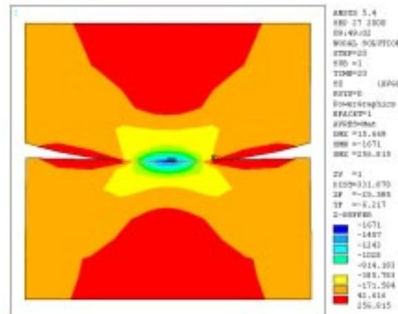
Fig. 7 Distribution of shear stress in plane  $x-y$
