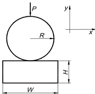
Fig. 2 Model of a cylinder and a flat elastic plate
