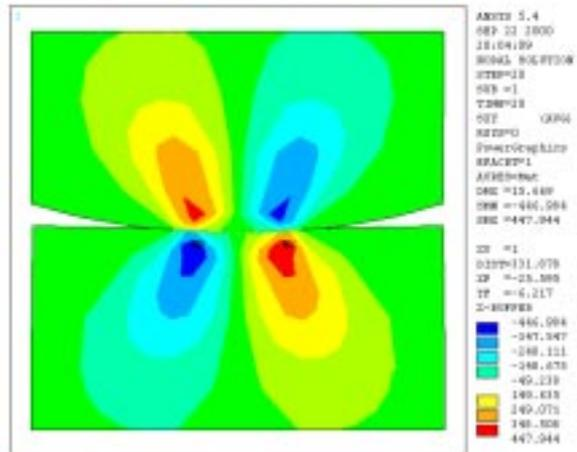
Fig. 5 Distribution of normal stress in direction of axis  $y$
