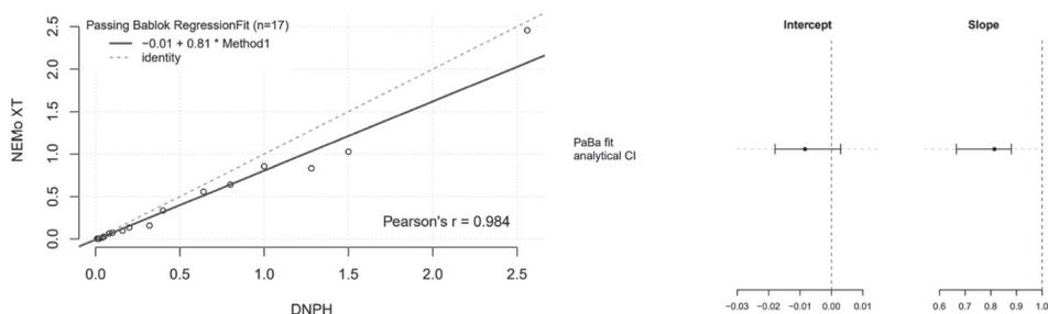
Figure 4. Graphical representation of Passing-Bablok regression between NEMo XT and DNPH
