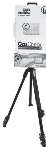
Figure 1. Monitoring devices: Proceas® (a), GasCheck (b) and NEMo XT (c)
