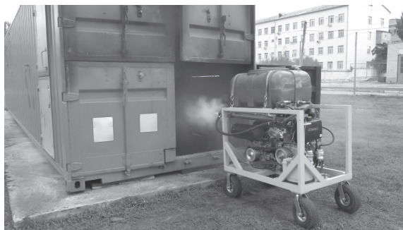
Figure 1. Fire extinguishing installation of a periodic pulsed action
