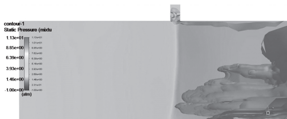
Figure 11. Distribution of the liquid in the barrel for a time period of 700 \mu\text{s} from the start of the action of the shock wave
