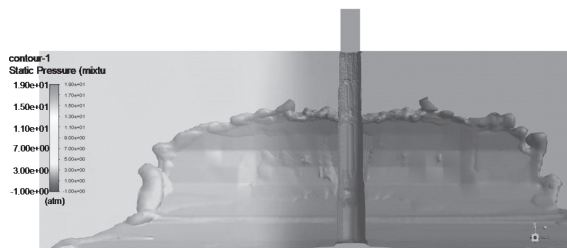
Figure 7. Distribution of liquid in the barrel for a time of 25 \mu s from the start of the action of shock wave
