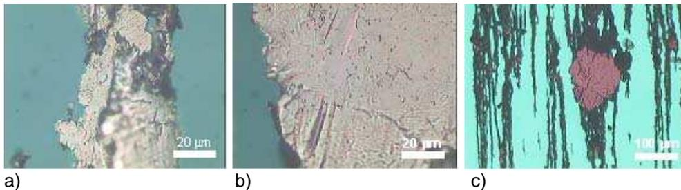
Very large wear particles and the presence of abrasive particles indicate the wear mechanism for uncoated and W-DLC coated gears is different. For the W-DLC coated gears, the wear probably started under the surface, while the prevailing wear mechanism for the uncoated gears is adhesive wear that started from the surface.
