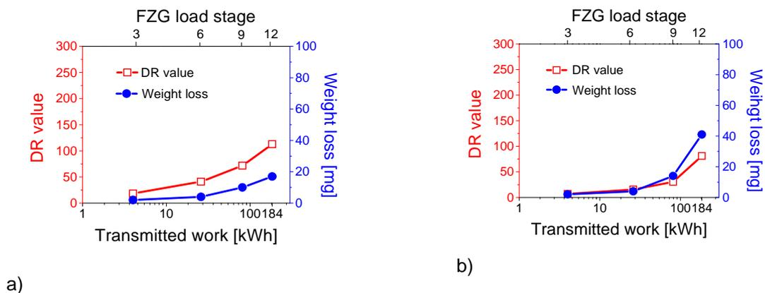
For the mineral oil formulation, the coating breakthrough started at the same time after 26 kWh of work transmitted, but visible damage was more severe. Developing scoring damage was observed during the subsequent runs for both oils. After the test, the pinion flanks were polished, and the W-DLC coating was totally worn out through at the root of the pinion. The wear results for W-DLC coated gears as
