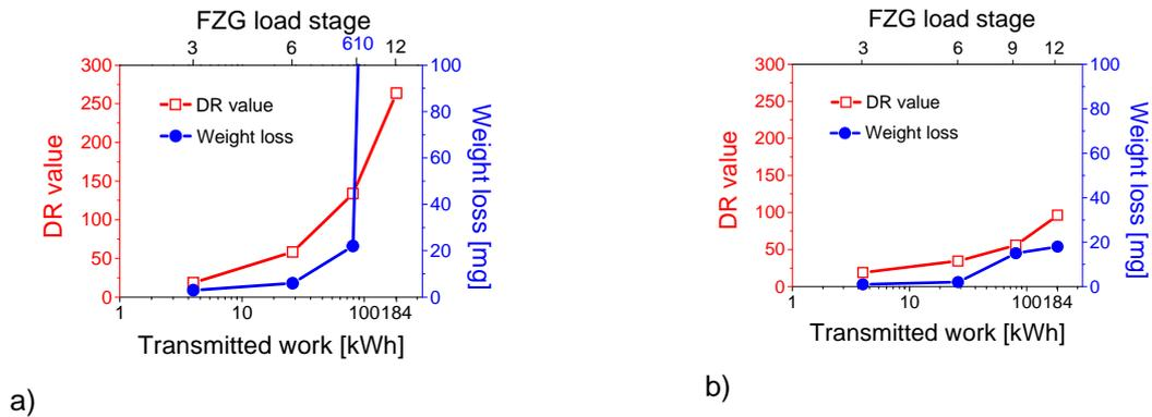
Figure 2: Wear measurements results for W-DLC coated gears: a) lubricated with the mineral oil formulation, b) lubricated with the ester formulation.
