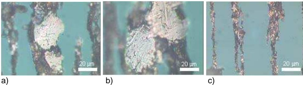
Figure 5: Entry region of the glass slide made from the ester formulation, magnified 500 times. a) uncoated steel gears; b) W-DLC coated gears; c) W-DLC coated gears – the largest cutting wear particles
