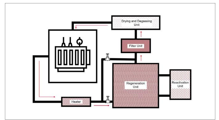
Figure 4. Graphical representation of Oil Reclamation
