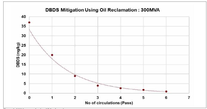
Figure 6. DBDS removal using Oil Reclamation
