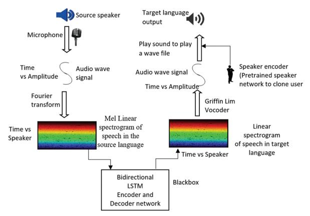
Fig. 2. Functional flow of STS conversion module
