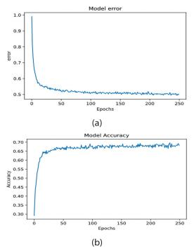
**Fig. 6.** Performance in terms of (a) error and (b) accuracy of the Bi-LSTM with attention in the proposed system
