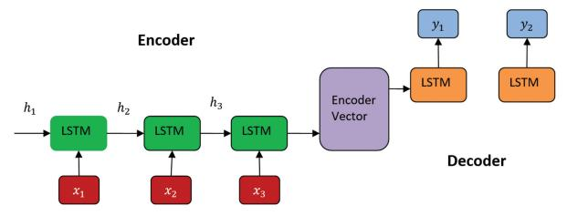
Fig. 3. LSTM based encoder and decoder network
