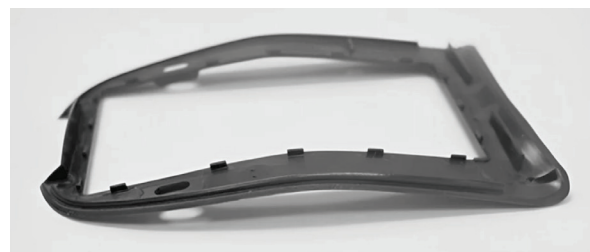
Figure 1 Example of moulded part warpage [1]
