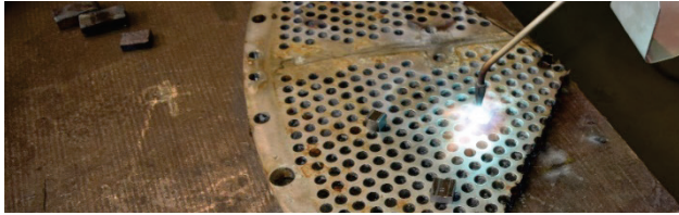
Figure 1 Spraying process using a gas flame with simultaneous fusing
