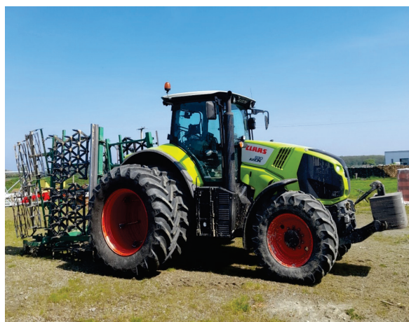
Figure 2 The tractor-machined aggregate used to perform the agrotechnical operation of closing the furrow
