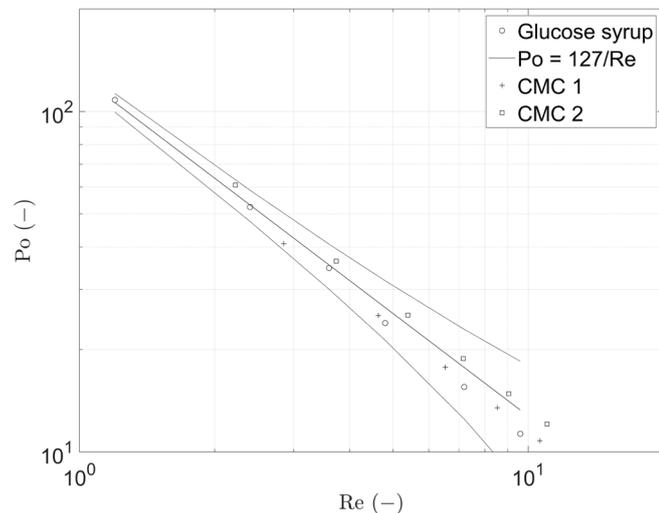
Fig. 5 – Comparison of the non-Newtonian and Newtonian power number results, converted using the obtained Metzner-Otto constant
