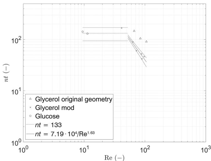
Fig. 2 – Dimensionless homogenization time characteristics with suggested regressions and a 95 % confidence interval
