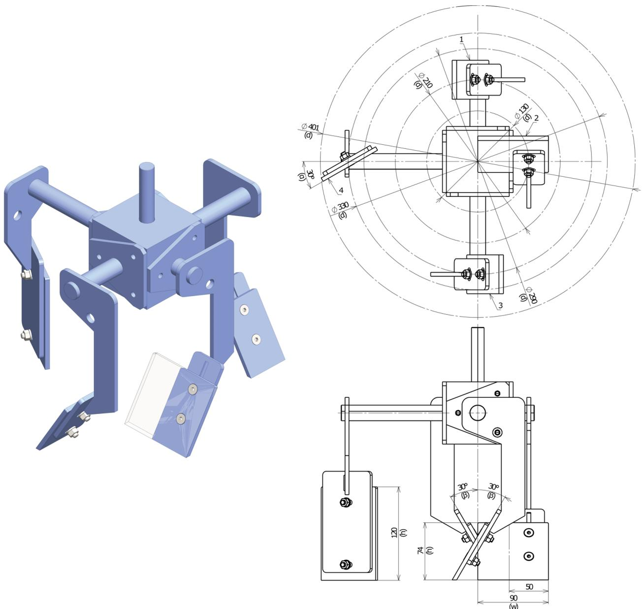
Fig. 1 – Isometric view of the paddle mixer assembly and sketch with the main dimensions
