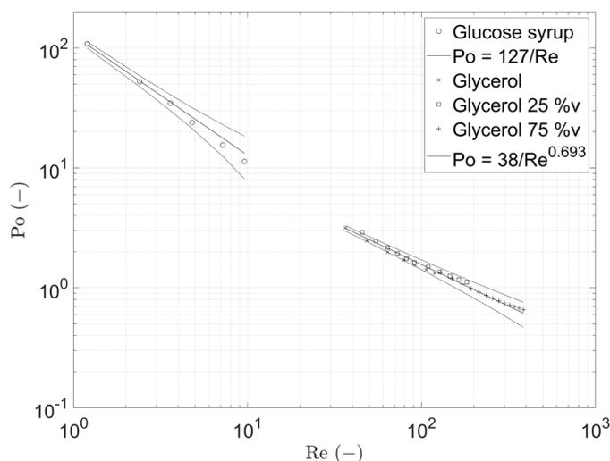
Fig. 3 – Power number characteristics for Newtonian fluids with suggested regressions and a 95 % confidence interval
