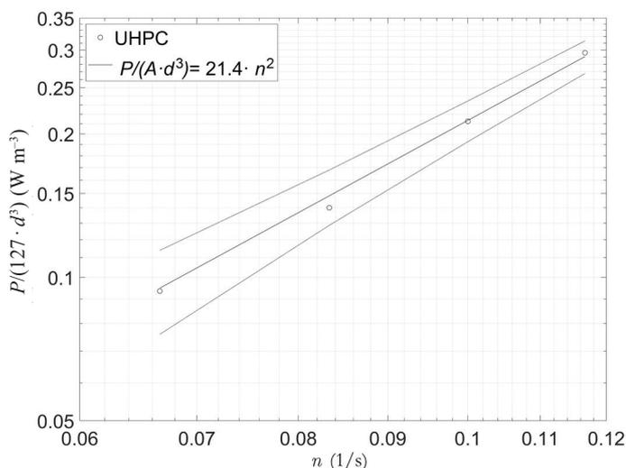
Fig. 6 – Result of the test measurement of the real UHPC mixture (both axes in logarithmic scale)
