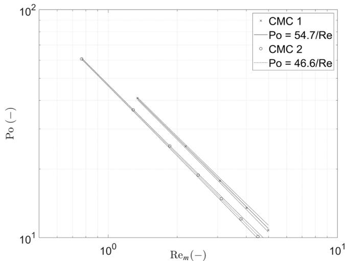
Fig. 4 – Plot of non-Newtonian results obtained using the Metzner-Otto approach with suggested regressions and a 95 % confidence interval
