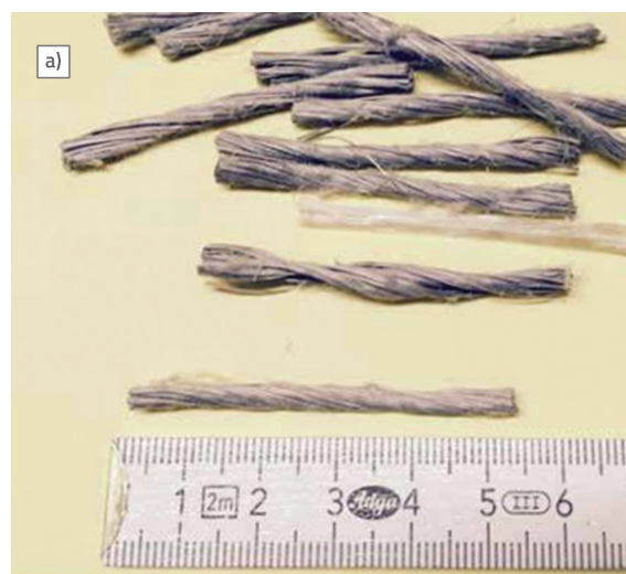
Figure 16. a) polypropylene fibre “AWP Forta Ferro”; b) concrete with fibres [3]
