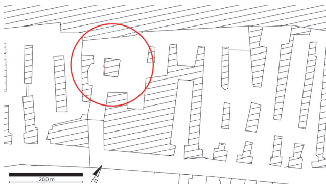
Figure 2. Site plan of the cellar system with the studied pillar; the hatched area refers to the support system
