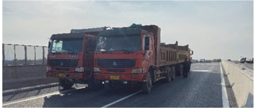
Figure 5. Phase of static testing of the bridge with 4 trucks
