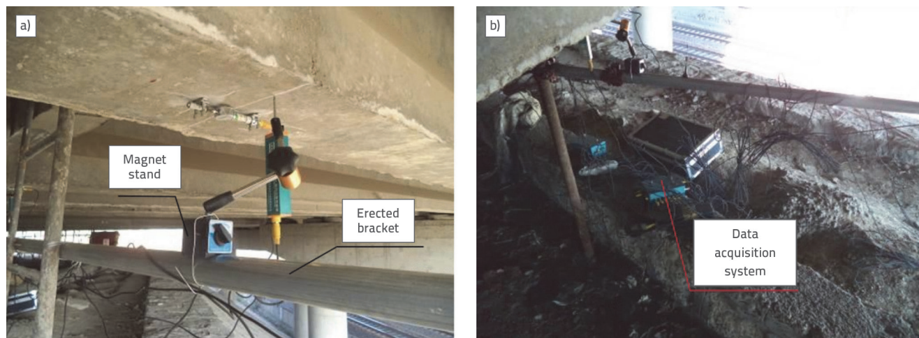
Figure 9. Setup for deflection measurement under the bridge: a) Setup method of displacement sensor; b) Layout of data acquisition system
