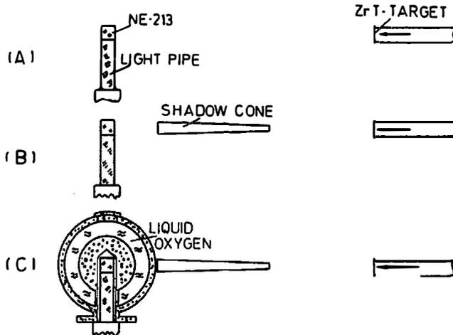
Fig. 2 — Geometry for the total elastic scattering cross section measurements.
