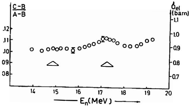
Fig. 3 — Measured cross section for neutrons scattered elastically from oxygen in the energy range between 14 and 19.5 MeV. The triangles indicate the energy resolution and the statistical error.
