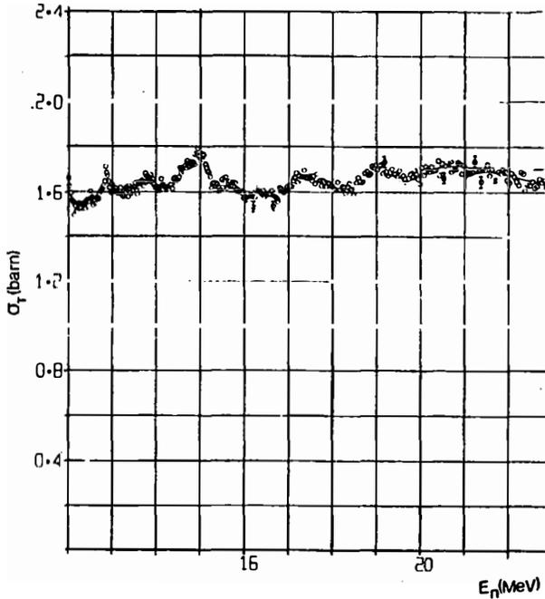
Fig. 4 — Total neutron cross section on  $^{16}\text{O}$  in the energy range between 12 and 22 MeV.
