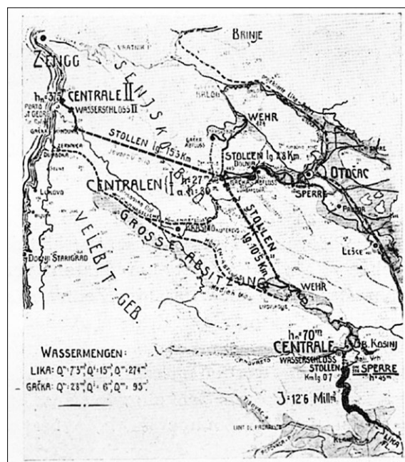
Figure 5: First hydropower potential utilization project on the Lika and Gacka - the precursor of the HPP Senj. Source: Theodor Schenkel, Karstgebiete und ihre wasserkräfte , Wien and Leipzig, 1912., 73.
