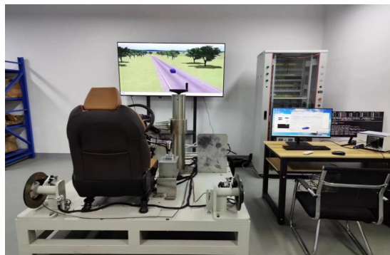
Figure 5 – Hardware-in-the-loop simulation platform (HIL)
