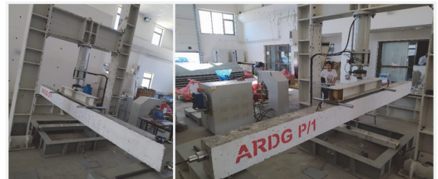
Figure 3 Test specimen and four-point bending test setup
