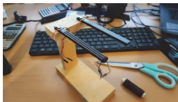
Figure 2 3D-printed beams attached to a rigid base
