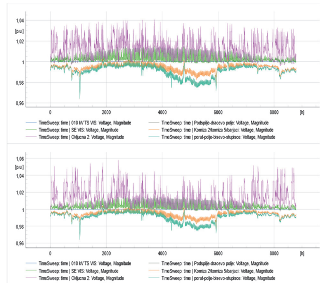
Figure 20 Island microgrid terminal buses voltage levels after PV + BESS + WECs with BESS integration at location 2 (up 7 Wavestars, down 238 Wavebobs)
