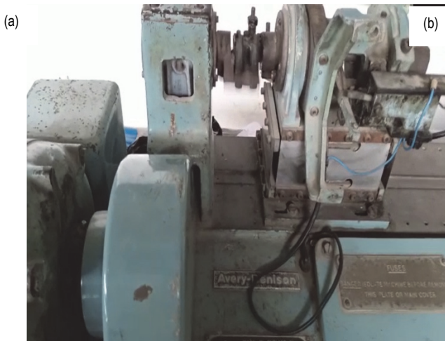
Figure 3 (a) Avery Denison Fatigue Testing Machine, (b) specimen specifications (Gauge length = 45.35 m, Final length = 52.52 m)
