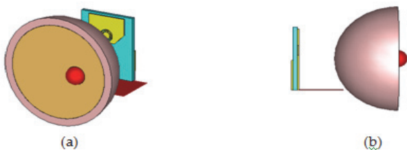
Figure 7 Textile Antenna placed behind the affected breast (a) Perspective View, and (b) Side view of antenna placed at 10 mm behind the breast
