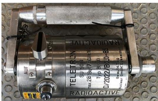
Figure 1. Exposure container Radioactive Teletron, SU 50N, type B (U), containing the radioactive isotope Ir-192
