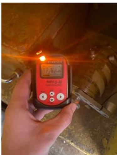
Figure 5. Checking the gamma meter during the measurement in the mini-bunker near the exposure container with the radioactive isotope Ir-192
