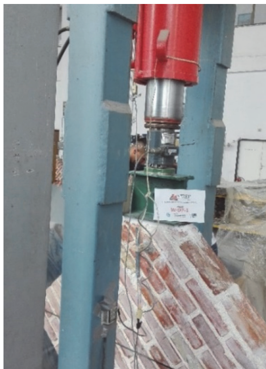
Figure 9. Test set-up for diagonal tensile strength test
