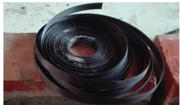
Figure 4. PP strip for bed joint reinforcement
