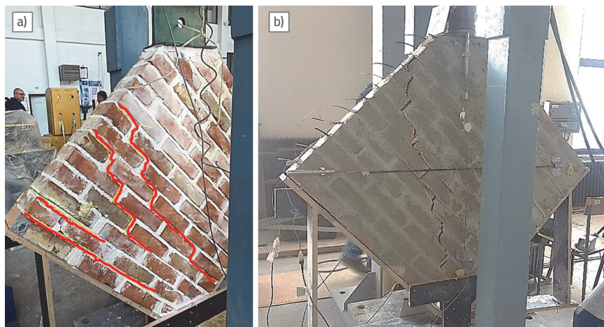
Figure 13. Typical failure mechanisms of masonry walls after diagonal tensile strength tests: a) URM panel (W-DP); b) SM panel (WS-DP-RPP)
