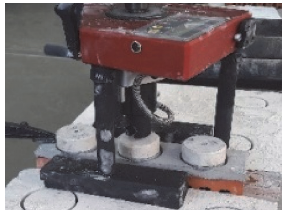
Figure 3. Pull-of tests on Reparatur mortar FS4
