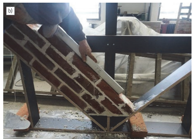
Figure 8. Plywood formwork and specimen construction for masonry diagonal tensile strength test: a) Drawing of the plywood formwork model; b) Construction of test panels
