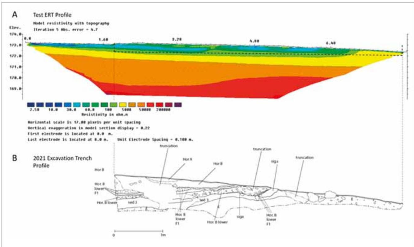
**FIGURE 6.** Ljubičeva Pećina (A)ERT profile with upper disturbance/intact sediment highlighted, (B) profile drawing of the same location after excavation (made by R. Becker).
