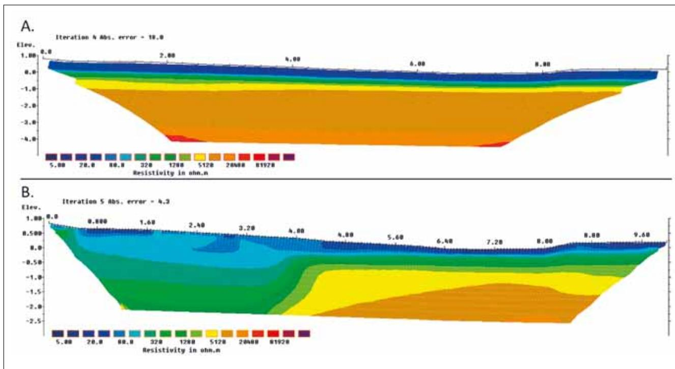
FIGURE 5. (A) Low & (B) high data density ERT profiles from Romualdova pećina (made by R. Becker).
