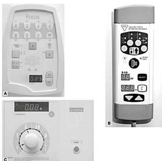
Figure 2. A,B,C) Different control panels of wall mounted X-ray device by several manufacturers
