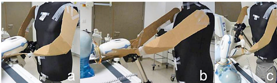
Figure 6. Positions of the handheld device and operator hands during acquisition: a) device parallel to the ground and close to the operator, b) device away from the body with fully outstretched hands (approximately 40 cm) and parallel to the ground, c) device perpendicular to the ground with partially outstretched hands
