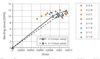
Figure 4. Stress–strain curves of the two sets of 30-mm-thick samples
