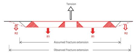
Figure 9. Schematic of the cross-section of the anchorage, highlighting the assumed and observed cones of the fractures. Therefore, each R1 value provided a tensile resistance of 1000 N. As the four holes were assumed to engage simultaneously, the total internal anchorage resistance was estimated using Equation (6).
