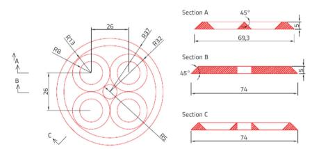
Figure 8. Plan and cross-sectional views of the anchorage element with dimensions in millimetres
