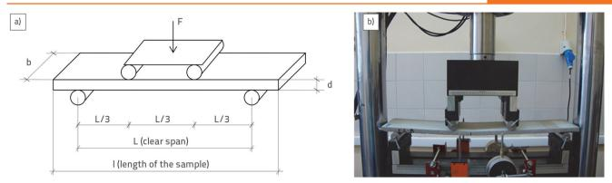
Figure 1. a) Suggested setup considering reference [9]; b) experimental setup and the four-point bending test of Sample 1-2-B
