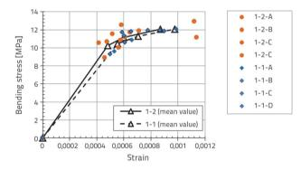
Figure 2. Stress-strain curves of the two sets of 10-mm-thick samples
