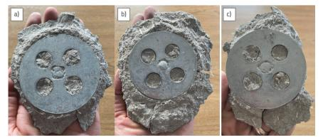
Figure 21. Close-up views of fractured anchorages in samples: a) sample 3; b) sample 4; c) sample 8
