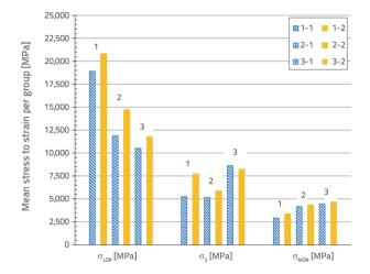
Figure 6. Estimated stress-to-strain ratios within the elastic and plastic stress-strain regions up to the respective stress limits  $\sigma_{\text{LOP}}$ ,  $\sigma_{\text{2'}}$  and  $\sigma_{\text{MOR}}$
