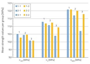
Figure 5. Mean bending strengths at the respective limits for each group of samples
