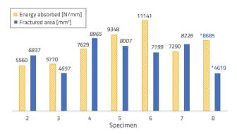
Figure 18. Comparison of the energy absorbed and fractured areas for each sample
