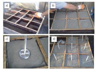
Figure 10. Production stages and embedment of an anchorage test sample
