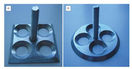
Figure 7. Prototype configuration of the anchor element: a) square formation; b) circular formation
