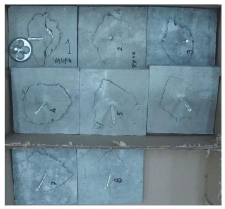
Figure 14. Plan view of the eight samples showing fracture patterns after the tensile failure tests
