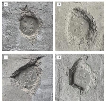
Figure 20. Crack patterns within the fractured base plates of samples: a) sample 3; b) sample 4; c) sample 5; d) sample 8
