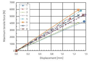
Figure 16. Linear and elastic force-displacement characteristics of the tested samples up to the highest stress limits
