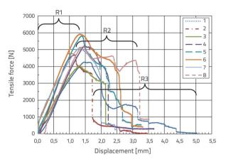
Figure 15. Force-displacement characteristics of the tested samples up to failure
