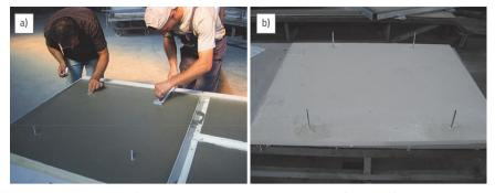
Figure 11. Embedment of square-based anchorage elements into fibre-reinforced concrete
