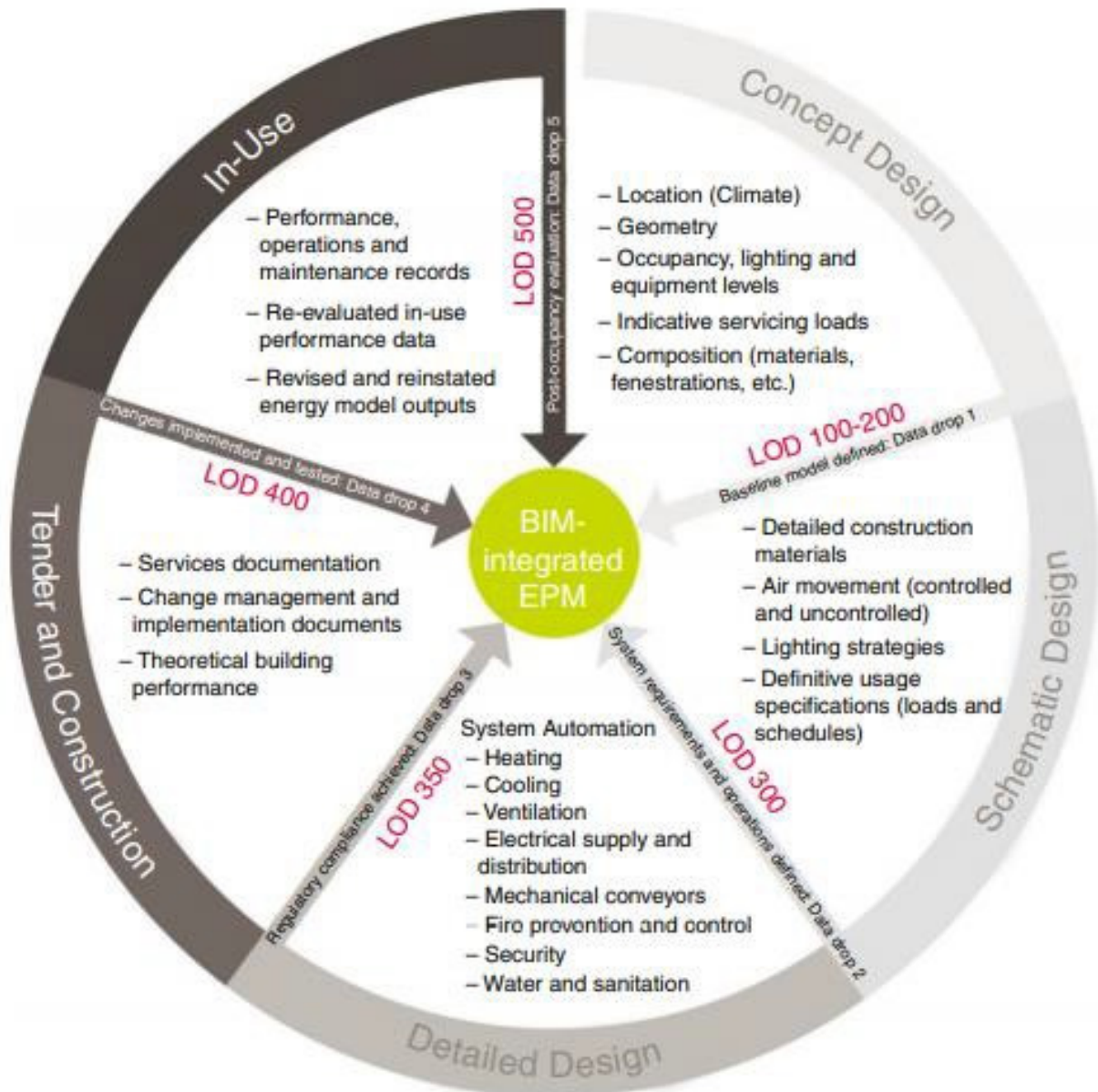
Fig. 3: Framework for BEM based on BIM capabilities for designing real estate projects. Source: Using BIM capabilities to improve existing building energy modelling practices (Gerrish et al. 2017). BEM, building energy modelling; BIM, building information modelling.
