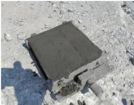
Fig. 7: Mortar samples for compressive and bending strength testing (left) and testing of bending strength (right).
