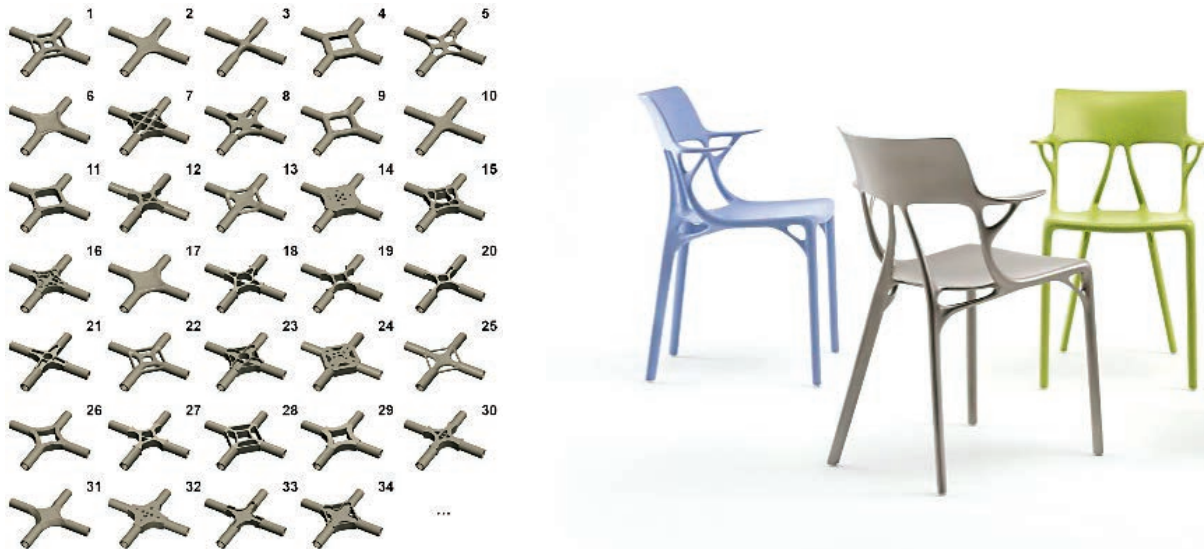
Figure 3 Left: Generative design of construction joint concept (Han et al. , 2022); right: AI Chair made with support of generative design tools (“A.I. chair Starck Kartel,” 2020)
