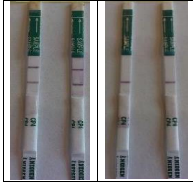
Slika 5. Vizuelno očitavanje rezultata prisutnosti GM sirovina u uzorku Figure 5. Visual interpretation of the results for the presence of GM materials in the sample
