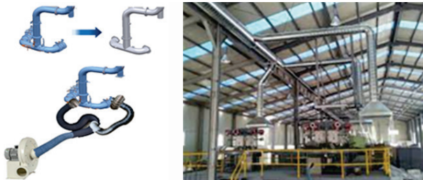
Figure 3 Diagram applying for the shape design of a multi-channel gas transfer pipe and VOCs collector.
