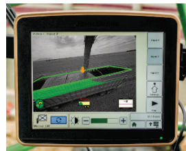
Figure 13 Active monitoring of trailer loading (Source: www.deere.com ).
