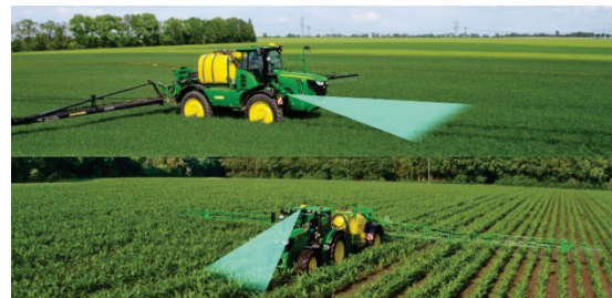
Figure 12 Camera locations in AutoTrac Vision system (Source: https://www.heavyquippmag.com )
