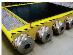
Figure 9 Transport platform with wheels (Source: www.arbeitsbuehnen-weiss.de )
