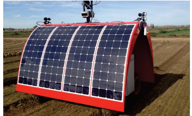
Figure 17 Ladybird autonomous vehicle (Source: https://www.abc.net )
