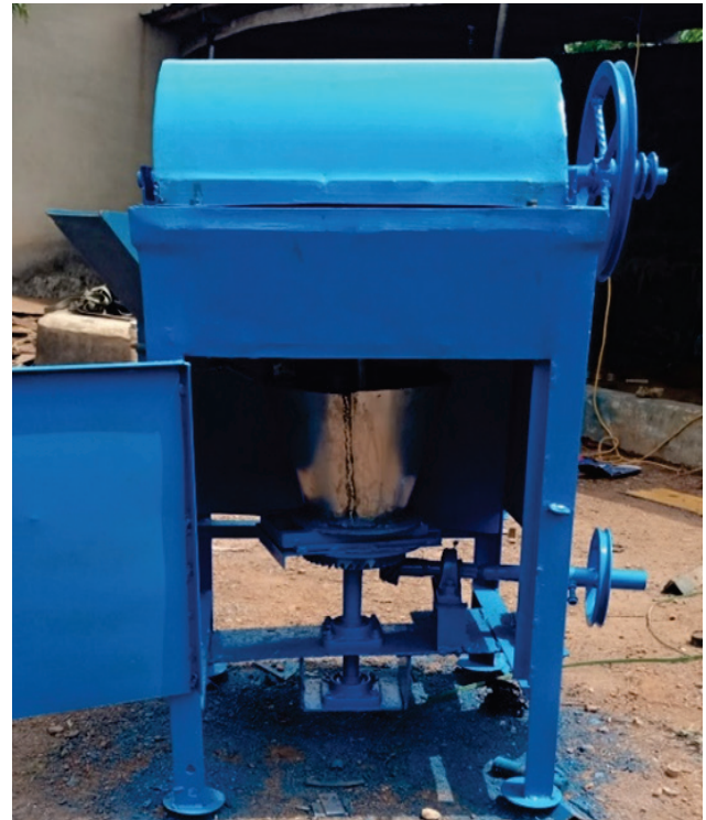
Figure 2 The developed vertical yam pounding machine
