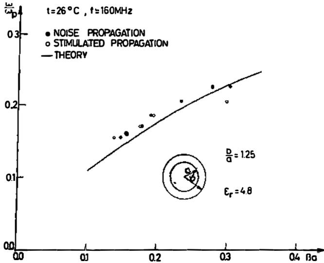
Fig. 7. Dispersion relation of a narrow band of the noise propagating in the form of surface waves, compared with stimulated propagation and theory.
