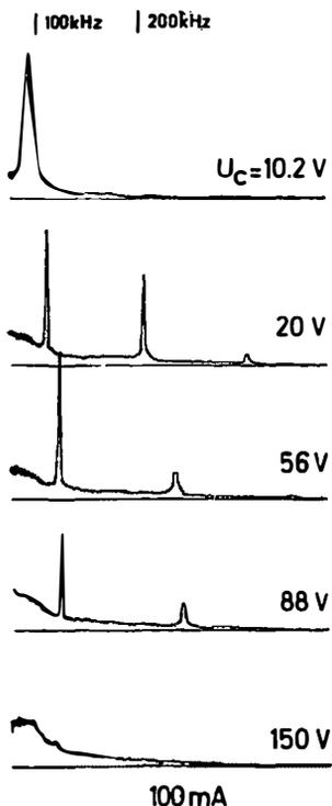
Fig. 3. Spectra obtained at 100 mA discharge current. The parameter is the cathode voltage drop.
