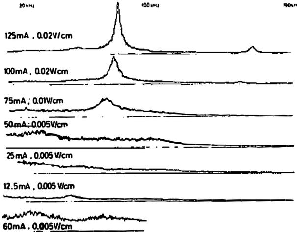
Fig. 2. Spectra of tube noise at various discharge currents, measured with a cylindrical probe in ion saturation.
