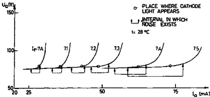
Fig. 5. Appearance of cathode light and high-frequency noise before saturation is reached.
