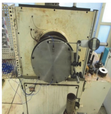
Figure 5 Representative DMF timing ring slipping torque machine
