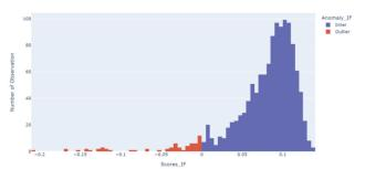
Figure 1 Outlier distribution based on the IF algorithm
