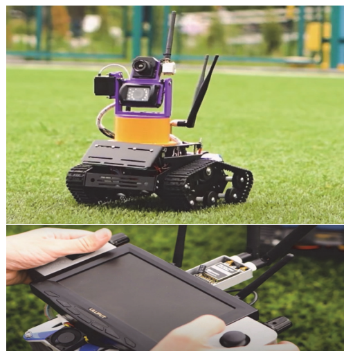
Figure 1 Mobile multi-purpose robotic platform for measuring thermal indicators of objects and remote control
