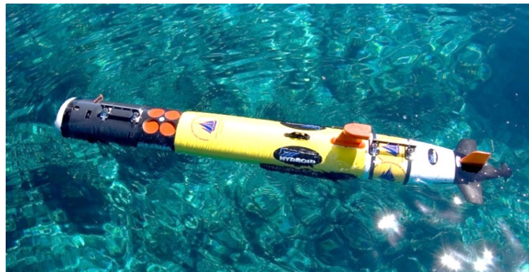
Figure 2. Small class unmanned underwater vehicle REMUS 100 (Source: Woods Hole Oceanographic Institution (WHOI), 2024a)
