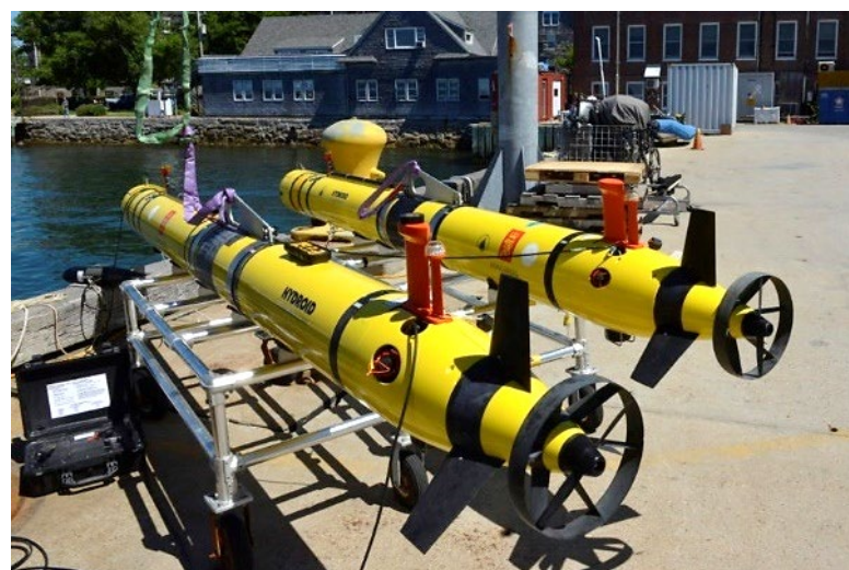
Figure 3. Medium-class unmanned underwater vehicle REMUS 600 (Source: Woods Hole Oceanographic Institution (WHOI), 2024b).
